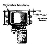
Figure 88. Print Suppression Magnet Adjustment
