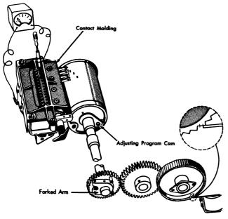
Figure 72. Program Sensing Contacts Adjustment
