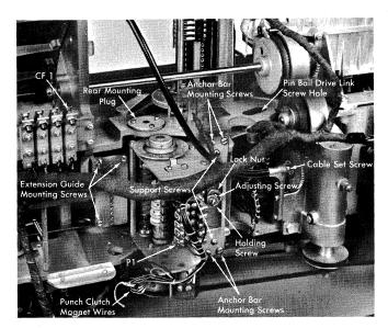
Figure 46. Punch Bed (Bottom View)
