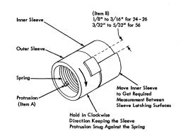
Figure 43. Punch Clutch Adjustment
