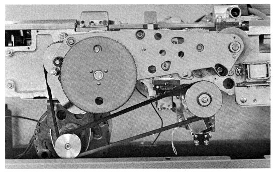
Figure 12. Reduction Gear Drive
