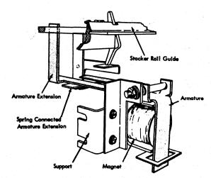
Figure 70. Offset Stack Magnet
