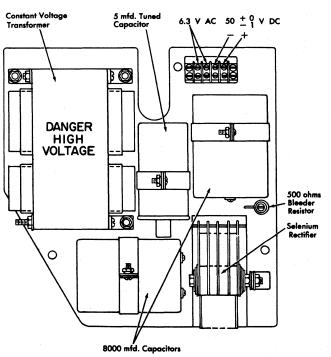
Figure 9. Constant Voltage Transformer Supply (Selenium)
