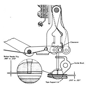
Figure 118. Reader Pin Interposer Clearance
