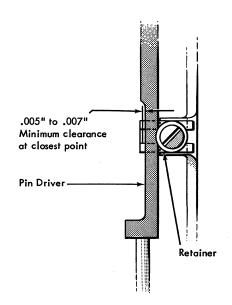
Figure 54. Pin Driver Retainer
