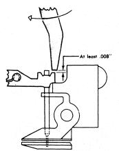
Figure 126. Contact Lever Clearance
