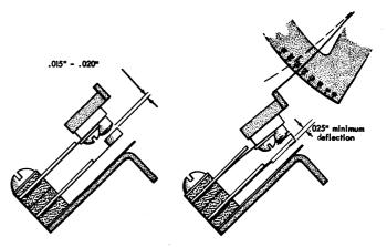
Figure 99. Detail Station Card Lever Contact
