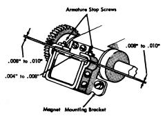
Figure 102. Auxiliary Transport Adjustment
