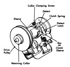
Figure 39. Error Retention Clutch
