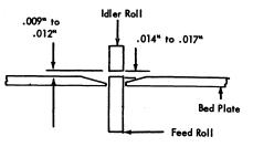
Figure 103. Auxiliary Feed and Idler Roll Adjustment
