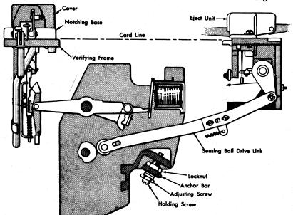
Figure 52. Verifier Drive Unit Timing
