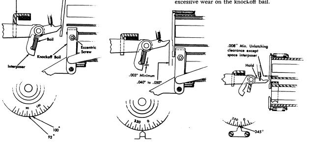
Figure 49. Interposer Relatching Adjustment Figure 50. Unlatched Clearance Check
