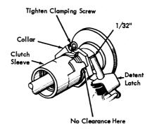
Figure 38. Clutch Adjustment
