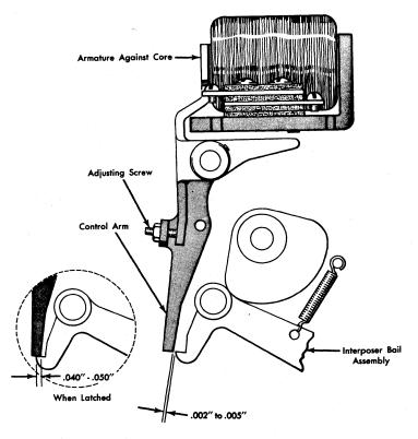
Figure 115. Control Arm Adjustment
