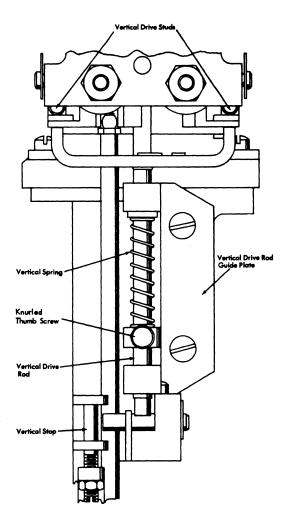
Figure 83. Vertical Drive Rod Assembly
