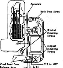
Figure 20. CF Latch Magnet Adjustment
