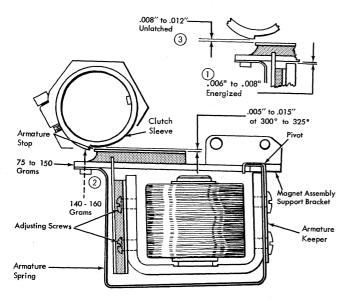
Figure 37. Punch and Verify Clutch Magnet
