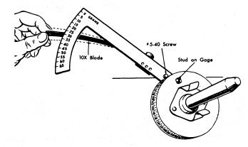
Figure 14. Friction Drive Adjustment
