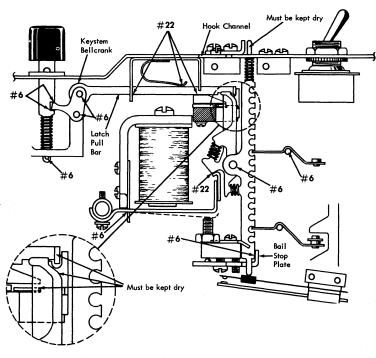
Figure 96. Keyboard Lubrication
