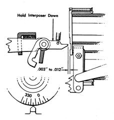
Figure 57. Interposer Unlatching Clearance
