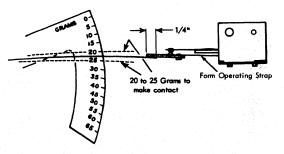
Figure 34. Interposer Bail Contact Adjustment (See Figure 127 for transfer-type contacts).
