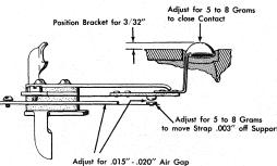
Figure 23. Card Lever Contact Adjustment
