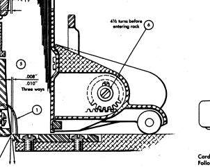
Figure 17. Hopper Adjustment
