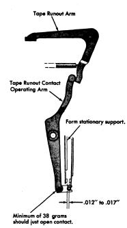
Figure 123. Tape Run-out Assembly
