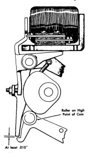
Figure 125. Latching Clearance
