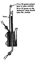
Figure 117. Sensing Contact Adjustment
