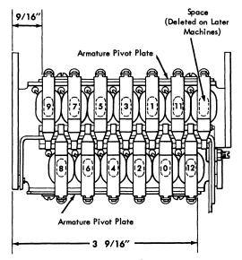
Figure 30. Armature Pivot Adjustment
