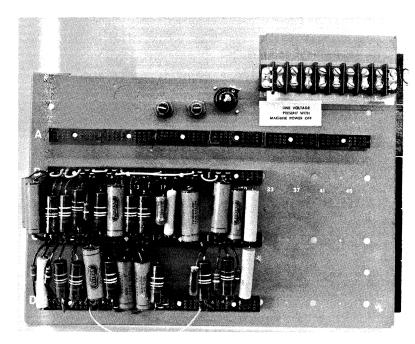
Figure 5. Power Supply for IBM 526
