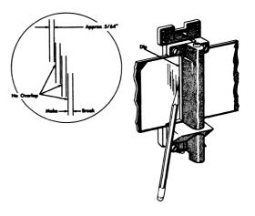
Figure 73. Program Sensing Contacts Adjustment
