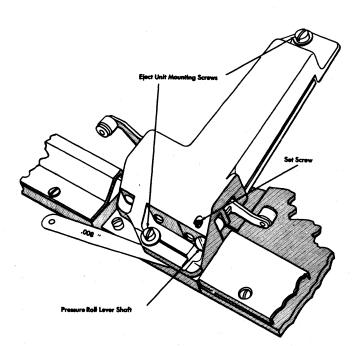
Figure 65. Check on Sensing Pin Contact Adjustment
