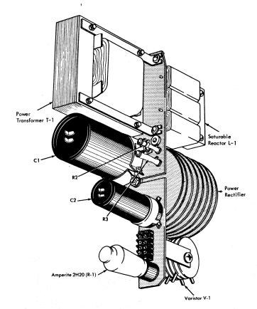
Figure 7. Saturable Reactor Supply
