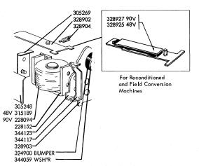
Figure 41. Punch Clutch Adjustment
