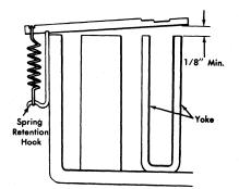
Figure 32. Armature Adjustment
