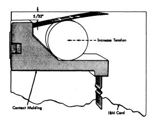
Figure 63. Sensing Pin Contact Adjustment
