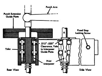
Figure 78. Punch Drive and Yoke Adjustment
