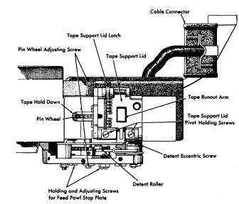
Figure 121. Tape Registration Adjustment
