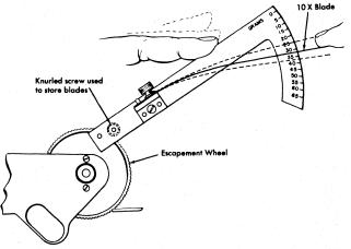
Figure 13. Friction Drive Adjustment
