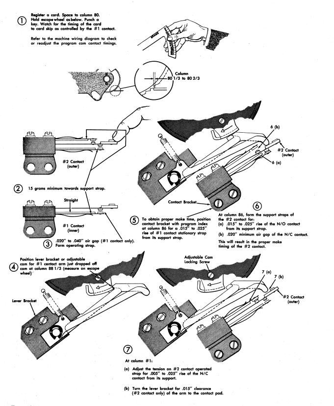
Figure 74. Program Cam Contact Adjustment
