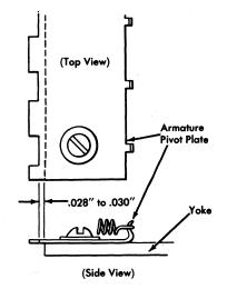
Figure 31. Armature Pivot Adjustment (Side View)
