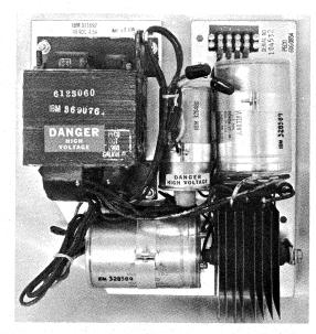
Figure 4. Power Supply for IBM 46-47, 65-66, and 834-836
