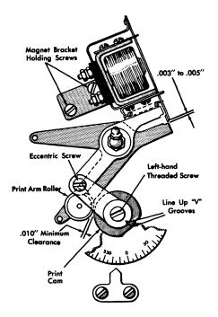
Figure 110. Print Magnet Adjustment
