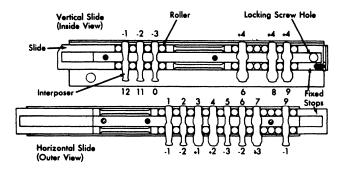
Figure 77. Print Interposer Assembly
