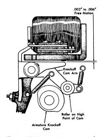
Figure 116. Magnet Armature Knock-Off
