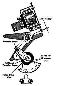
Figure 60. Notch Drive Unit
