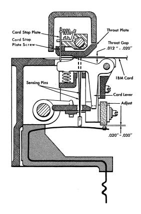
Figure 64. Pin Sensing Adjustment
