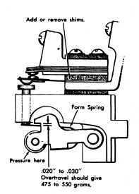
Figure 44. High-Speed Circuit Breaker
