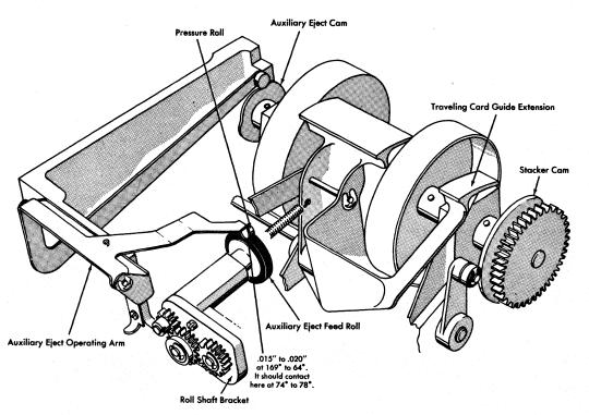
Figure 100. Auxiliary Eject Mechanism
