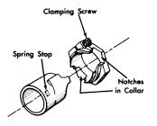
Figure 40. Clutch Sleeve and Collar
