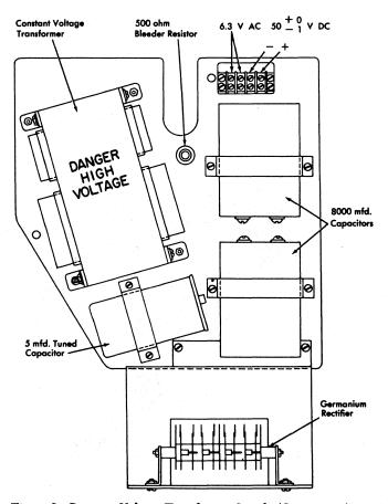
Figure 8. Constant Voltage Transformer Supply (Germanium)
