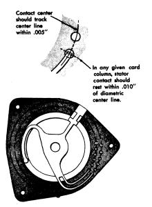
Figure 113. Card Column Emitter Adjustment
