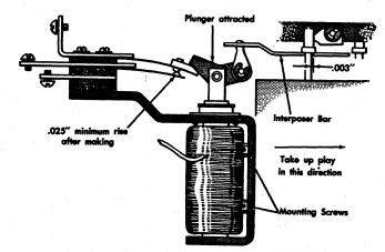
Figure 61. Last Column Notch Solenoid
