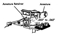
Figure 69. Offset Stack Magnet Adjustment
