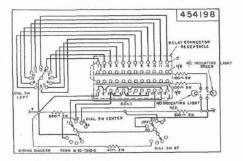
Figure 30B. Testing Device Wiring Diagram
