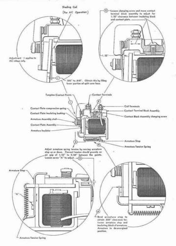
Figure 14. IBM Unit Type Relay
